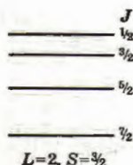
Fig. 38. Example of an Inverted Term ^4D . Corresponding to the interval rule (see p. 178), the separation of the components increases from top to bottom, contrary to a normal term.
