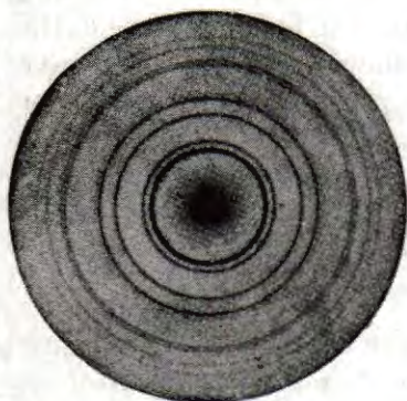
Fig. 14. Photograph of Electron Diffraction by a Silver Foil. Electrons with a velocity of 36,000 volts, corresponding to a wave length of 0.0645 Å, were used in the experiment [after Mark and Wierl (49)].
