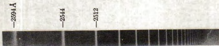
Fig. 2. Absorption Spectrum of the Na Atom [Kuhn (42)]. The spectrogram gives only the short wave-length part, starting with the fifth line of the principal series. The lines appear as bright lines on a dark continuous background, just as on the photographic plate.
