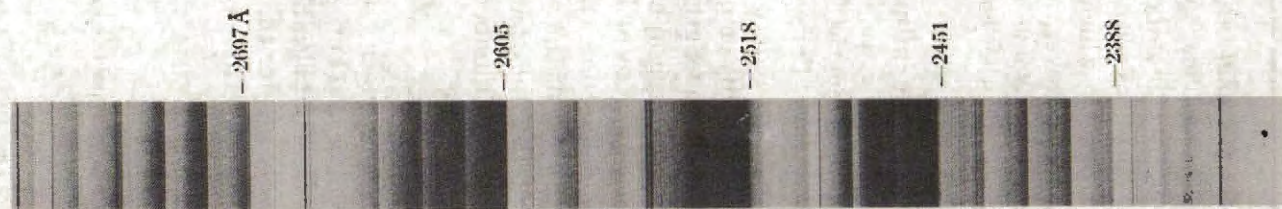
Fig. 7. Band Spectrum of the PN Molecule [Curry, Herzberg, and Herzberg (43)].
